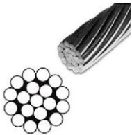
Stainless Steel 316 Cable Ø3/16", 1X19 Construction
